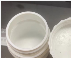
Aluminum foil missing
