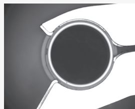
Through-holes in the bottle neck
